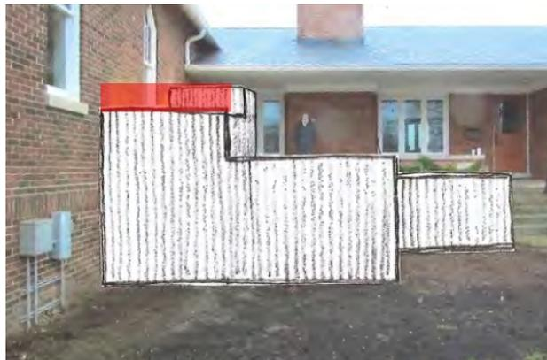
The above graphic will assist visualizing this but is not intended to represent a formal plan. The recommendation is to increase the height of the panel (represented in red) to avoid the need for multiple elevations of fence.
